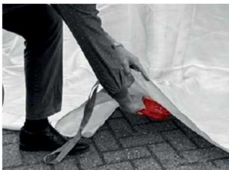
Place/throw the aerosol unit under the car/blanket, as close to the battery as possible
