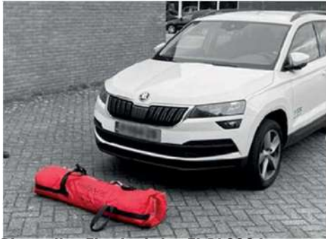
Place the Fire Isolator FI-BL0906 blanket in front of the car
