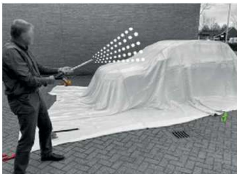
Spray a water mist over the car/blanket - 1
