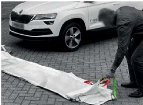
Pull half the blanket over half the car using the (green) loops
