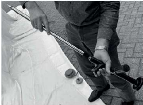
Assemble the water mist lance
