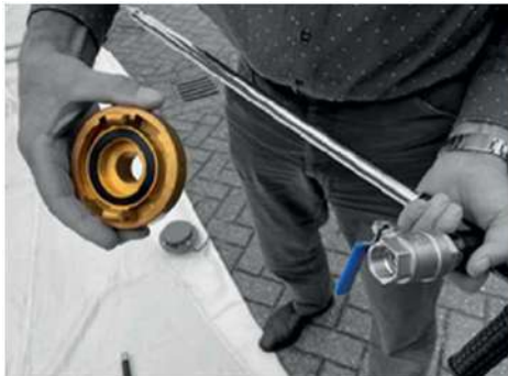
Ensure the correct fire hose connection
