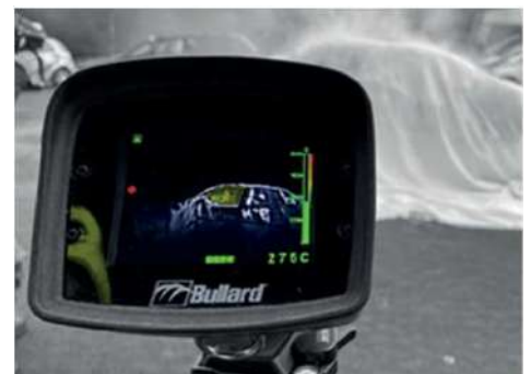
Monitor the temperature development of the fire using a thermal camera
