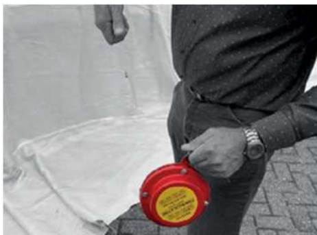
Activate the aerosol unit by pulling out the cord
