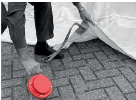
Place/throw the aerosol unit under the car/blanket, as close to the battery as possible
