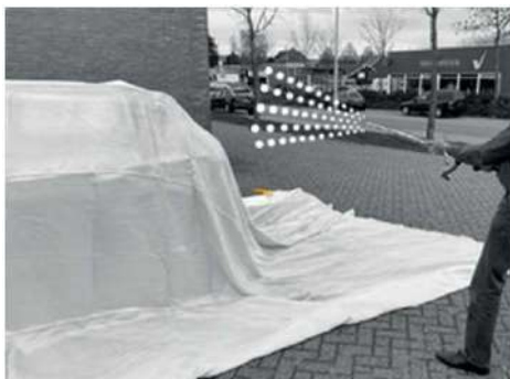
Spray water mist over the car/blanket - 2
